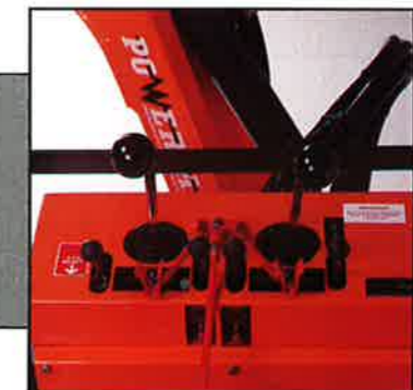
TWO LEVER CONTROL OF DIGGING FUNCTIONS.
