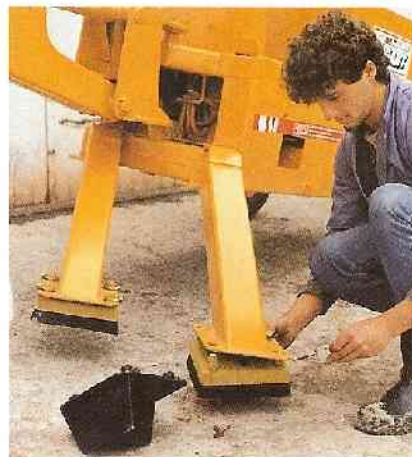
Steel pads can be replaced by rubber pads quickly without tool. Surface protection
